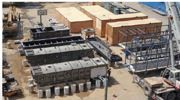
34 tanks and process vessels for a uranium SXEW plant -Technip/Areva - Canada
